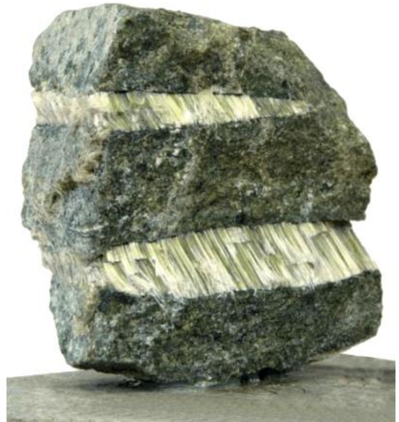
Serpentinite rock with chrysotile mineral fibers
