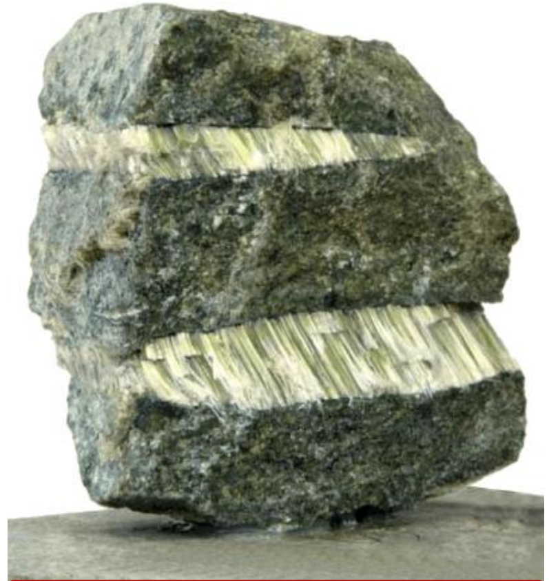
Serpentinite rock with chrysotile mineral fibers
