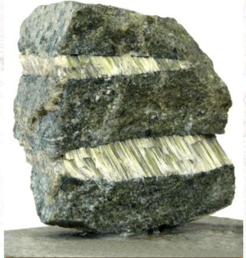
Serpentinite rock with chrysotile mineral fibers
